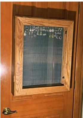
In addition, the whole cabinet was designed to be securely attached to the outside of a closet door, using hangers affixed near the top of the back panel and rubber bumpers along the bottom of the panel to prevent marring the finish of the closet door.
